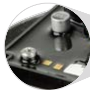
Epoxy filled electronics
