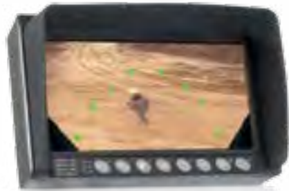
Camera setting: Graticule. This option shows a graticule for a Rearview camera on the monitor.
