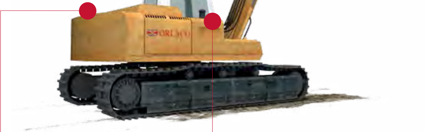
RadarEye setting: Transparent visualization of the radar-zones on the display. (standard preset setting)
